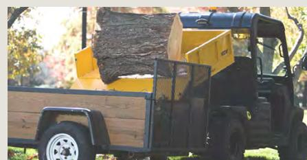
**DUMP** - LeveLift bed technology also enables loads to be dumped at any height or distance along its arc of motion, providing owners more options for where and how their cargo can be unloaded.
