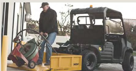
**LOAD** - Flip the switch and the LeveLift bed technology brings the cargo box up, back and down, enabling you to load at ground level or at any point along the bed's arc of motion.
