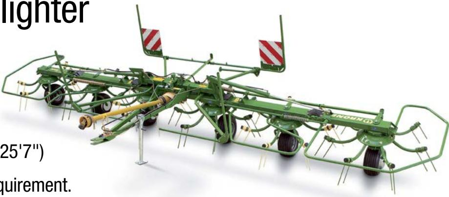
Running on the middle wheels when in transport, the machine does not mount in the tractor's three-point linkage – which is ideal for smaller tractors with lower front axle load and lift capacities.
