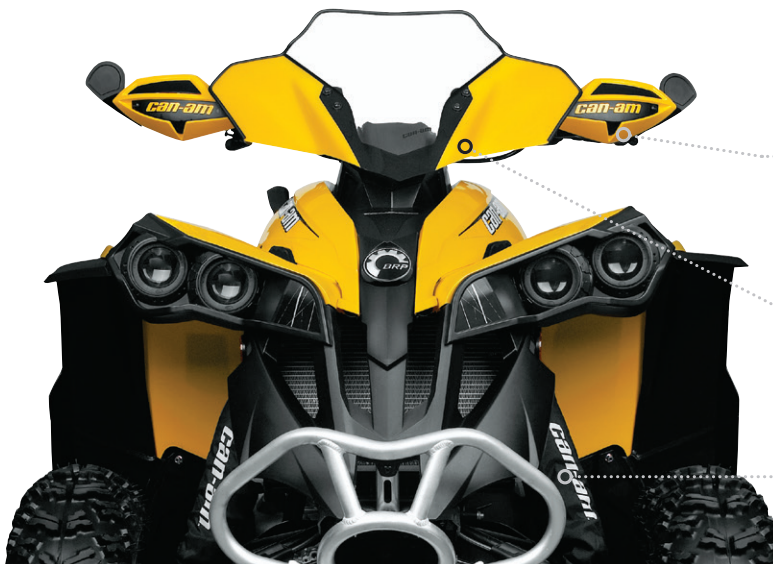
MUDGUARD KIT Integrated extended fender flairs for sporty look and full body protection from dirt and water.
