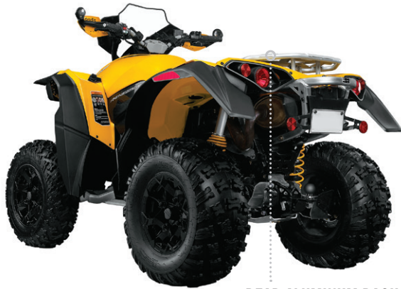
REAR ALUMINUM RACK 30-lb (14 kg) capacity. Compact, lightweight aluminum construction.
