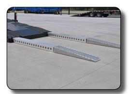
The Dual Ramps are Supplied as a Standard Feature. You Have the Flexibility of Using One or Two Sets to Achieve 5° Load Angle.
