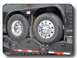
Adjustable Wheel Well Pockets with Five Different Positions Minimizes the Clearance Under the Bus as well as Lowers the Overall Height.
