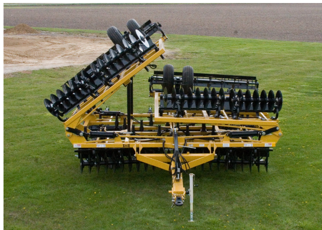
The 35' and 40' Tilloll has a stack fold system with a transport height of 13'0"(35') and 13'9"(40') and transport width of 17'9".
