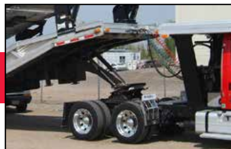
Tilt Cylinder - Major Steel Components Powder Coated
