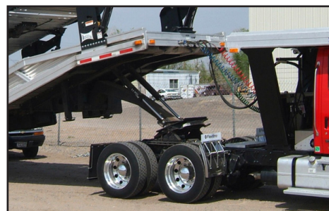
Tilt Cylinder - Major Steel Components Powder Coated
