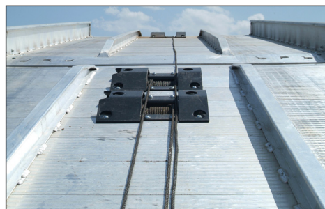
One Winch per Vehicle Upper and Lower Deck
