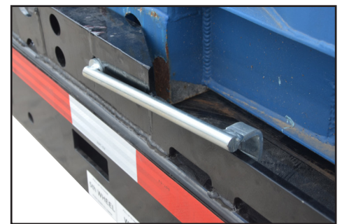
• Container Lock Down Side Pins
