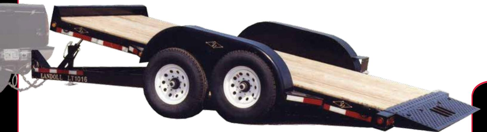
A 6"channel iron frame under the main frame for superior strength. A solid formed 6" height headboard for protection.
