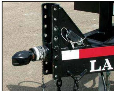
The hitch adjusts from 12" to 24" vertically.
