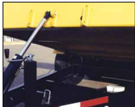
The cushion cylinders tilt the bed to ground position and back to transport position smoothly.
