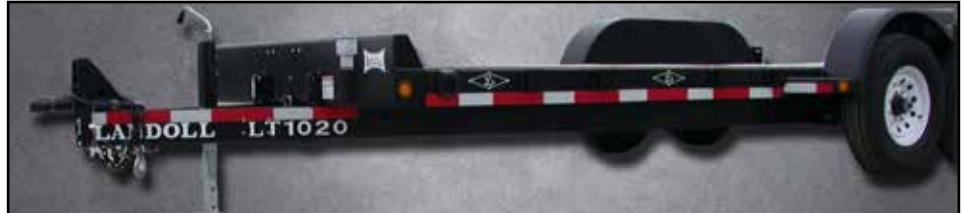
A 6" channel iron frame under the main frame for superior strength. A solid formed 6" height headboard for protection. (Stake pockets shown for optional removable sideboards)
