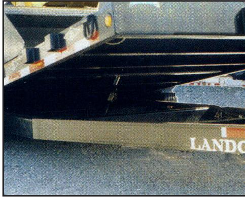
The Landoll tilt control system and the  $2\frac{1}{2}'' \times 16''$  cushion cylinder can hold the deck in a tilted position or smoothly return the deck to transport position.
