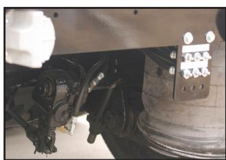
Manufactured by Landoll Corporation, the centralized lube system provides remote grease zerks to each individual greaseable point on the trailer undercarriage including the slack adjusters and camshaft bearings, which both require regular grease for optimum performance. Maintenance time and costs are reduced significantly.
