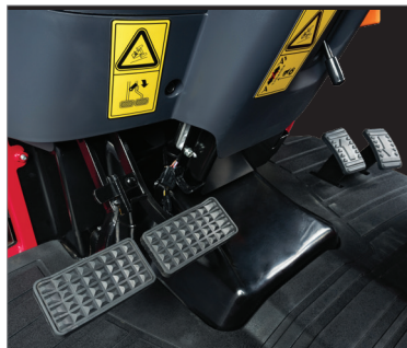
DUAL BRAKES OFFER A TIGHT TURNING RADIUS.
