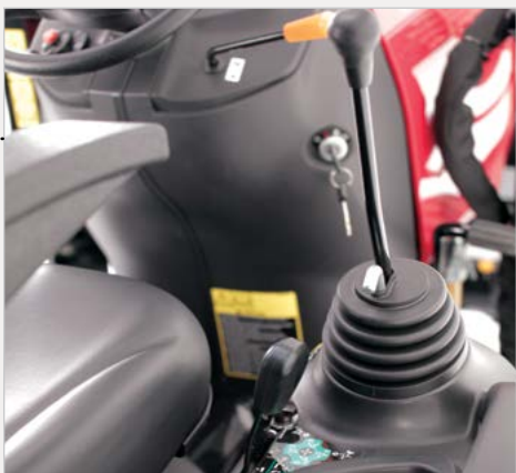
Work comfortably with armrest-mounted loader control lever, while True Position Control lever (below joystick) delivers precise operating height of rear implements.
