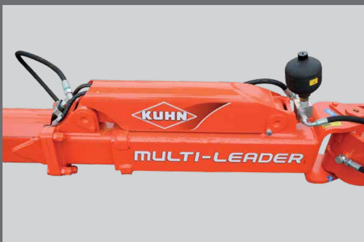
3. Offset : by mechanical tie rod or hydraulic cylinder (as an option) makes the inter-tyre adjustment from 1.15 to 1.60 m. A gauge visible from the tractor cab facilitates setting precision.
