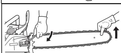
5. Pull the chain around the bar by hand. Loosen the adjustment if you feel tight spots.
