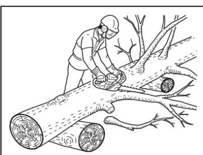
Don't cut with the saw overhead or aligned vertically with your body. If the saw should kickback, you may not have enough control to prevent possible injury.
