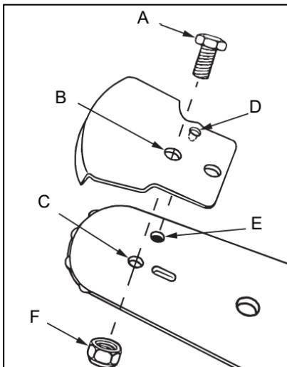
**Guide Bar and Saw Chain Removal and Installation**
