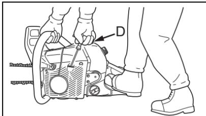
6. After starting the engine, pull front hand guard towards the operator immediately (chain brake unlocked position).
