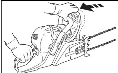
3. Hold the bar nose up, and turn the adjuster toward (+) until chain contacts underside of the bar.
