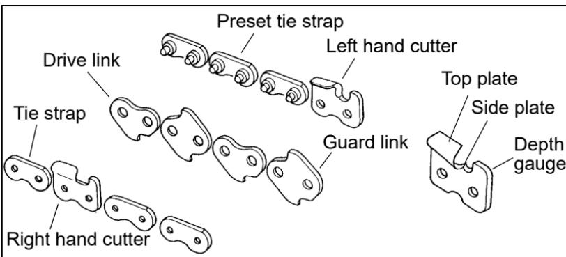
Important points for proper maintenance of saw chain:
