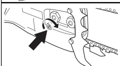
4. Tighten nuts with the bar nose held up.
