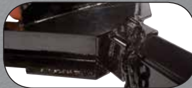
C channel frame construction for extra strength
