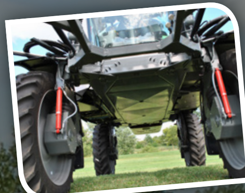
HYDRAULIC TRACK ADJUST The RUBICON axle track width can be adjusted, on-the-run, from 3,0 m to 4,0 m The integrated air-ride suspension provides superior ride and performance.
