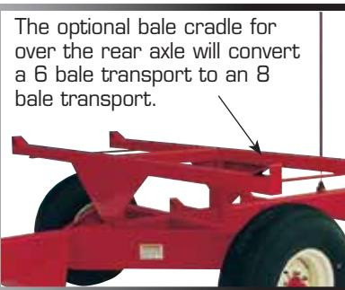
Bale cradle arms are  $3/16"$  square tubing, reinforced with gussets, and tied together with a flat metal strap to keep them from spreading.
