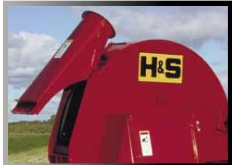
The hinged blower outlet assembly is removable for easy inspection and maintenance of the cupped paddles.
