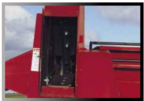
Cupped replaceable blower paddles mounted in front of the rotating side backplate provide unsurpassed free movement of material from the 30° angle feed auger without any loss of momentum.
