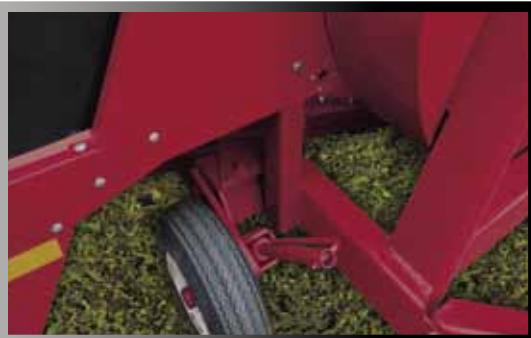
A built in crank is provided for each wheel to allow for height adjustment for different sized forage boxes and also allows you to raise and lower the blower for transport. Transport wheels are equipped with bearings, not bushings.
