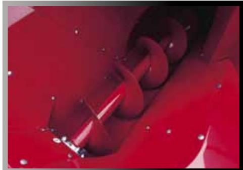
The 12 inch diameter feed auger is positioned at a 30° angle to the blower which moves material freely into the blower for maximum capacity.
