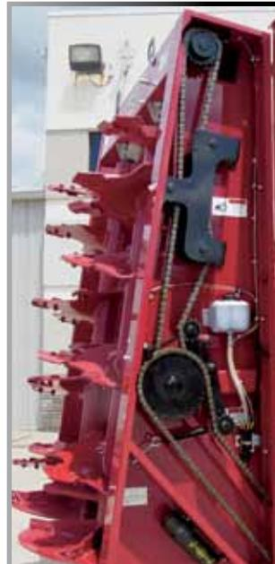
An Auto-oiler for the vertical beater drive chains is standard equipment.
