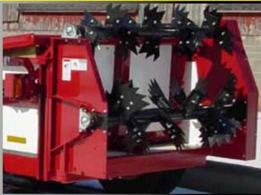
Horizontal beater models feature a top beater as standard equipment and are shear bolt protected at the front pto assembly.
