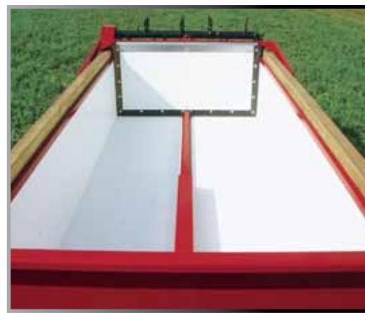
All Hydraulic Push models use solid virgin grade poly with UV inhibitor, for the floor and sides allowing less friction.
