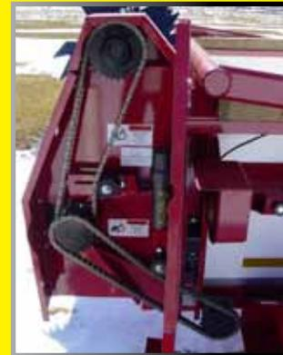
The beaters are driven by the HP's unique center drive system. #80 chains are used for strength and long life. Easy open shields makes lubing of chains easy.
