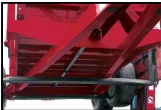
Heavy duty rectangular tubing is used for the pole to ensure strength and long life.
