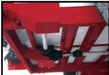
The HP's PTO beater drive system consists of a straight shaft off the PTO underneath the center of the manure spreader to an angle gearbox in the rear, and over to the beater drive sprocket.
