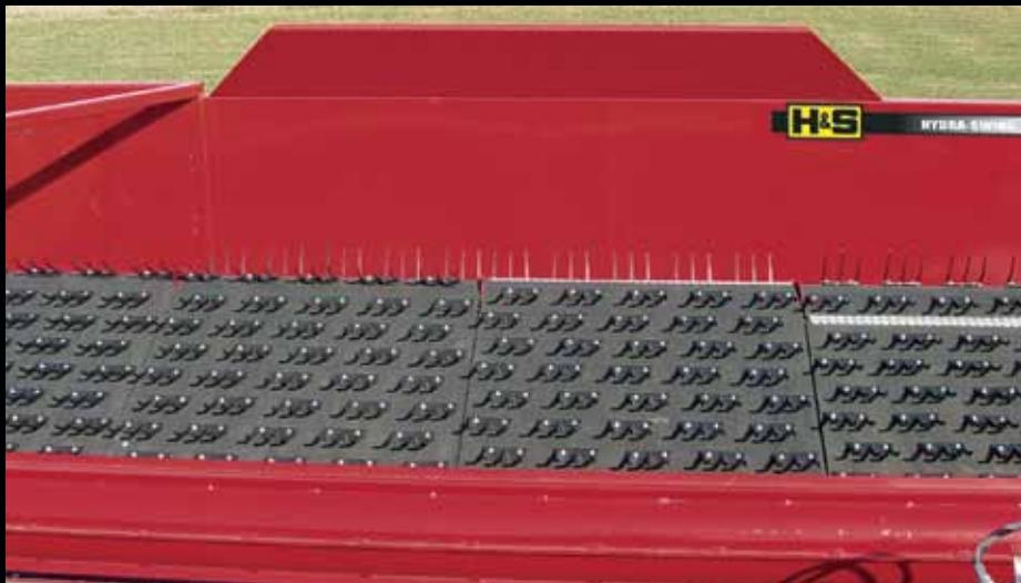
Replaceable three prong plastic teeth handle the crop gently and the high rear panel prevents spillage over the back.
