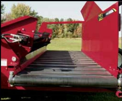
A heavy duty 42" wide, ribbed cross conveyor easily accommodates the massive flow of material. A cross conveyor shut-off is optional on all Hydra-Swing Mergers.
