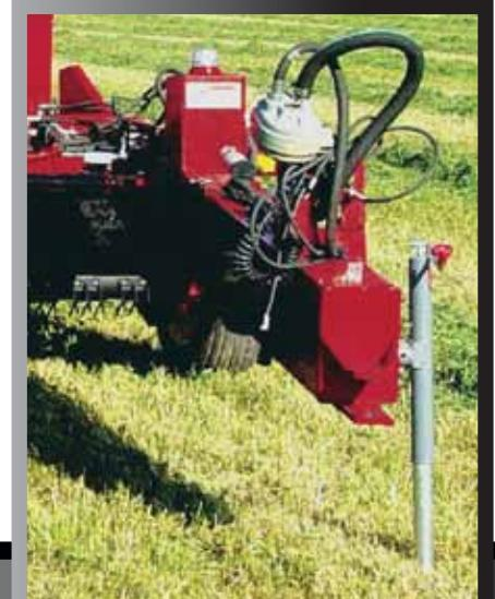
An optional self contained hydraulic drive kit with P.T.O. pump can be installed on the H&S Hydra-Swing Mergers. This feature allows tractors with a minimum 5 G.P.M. hydraulic capacity and 1 remote to operate the merger.
