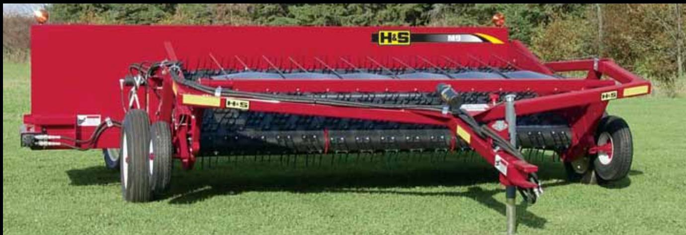
Capacity on an H&S Merger is second to none. Built with strength and quality, H&S Mergers can handle the tough field conditions and provide a smooth, clean pickup of material! The M9 Merger has a 9' pick-up head and a cross conveyor width of 42".
