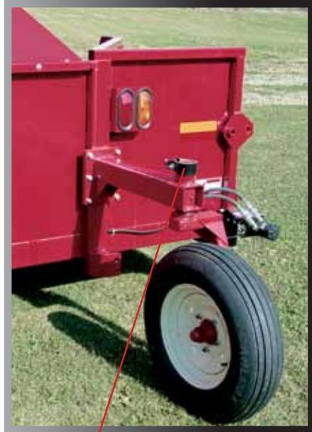
The rear swivel tail wheel has a brake assembly that can easily be tightened by a single bolt for severe field conditions or transport.
