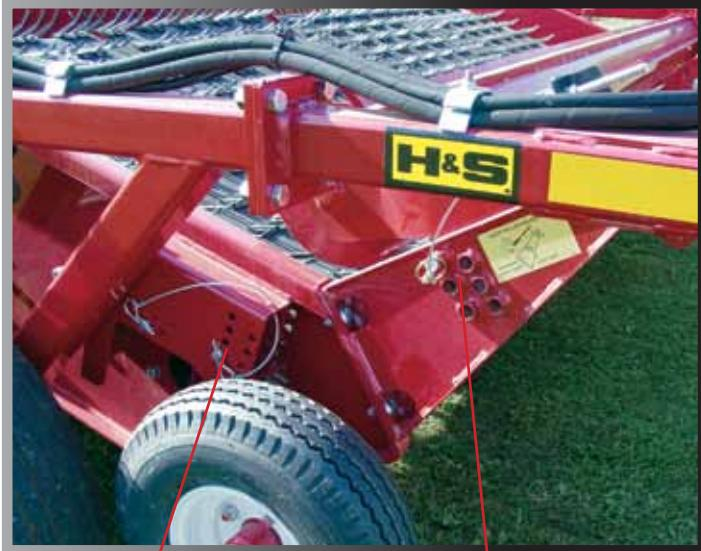
The gauge wheels and Hydra-Swing Crop Roller are easily set to crop conditions just by removing and replacing the pins in the desired setting. The Crop Roller is standard on Hydra-Swing models and optional
