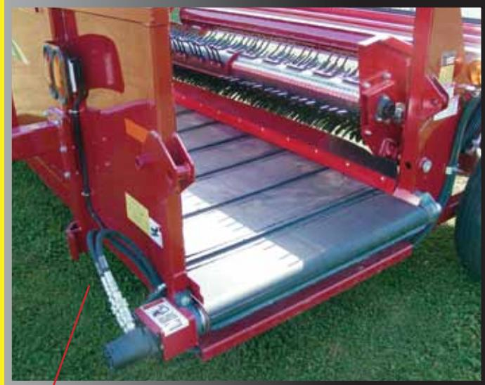
By switching the 2 easy quick disconnect hoses around, you can change from right side merging to left side merging or inverting with the optional inverter shield.
