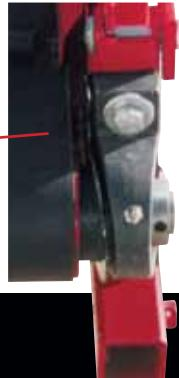
H&S Mergers feature an anti-wrap guard (patented) on the cross conveyor bearings to protect against material wrapping on the shafts and destroying bearings.
