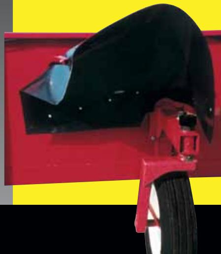
Storage for the inverter shield is out of the way behind the machine. The optional left side inverter shield can easily be mounted on either the M9 or the Hydra-Swing Mergers.
