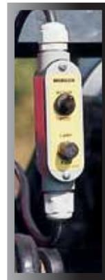
A tractor mounted electric control box directs hydraulic oil flow to swing the tongue or raise and lower the pickup on the Hydra-Swing Mergers.
