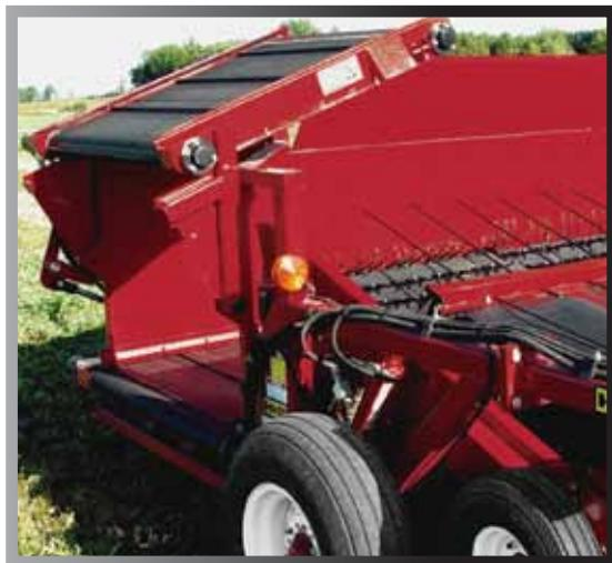
Hydraulically folding the optional 2', 4', or 6' extension out of the way, and turning the hydraulic valve to the off position, the Hydra-Swing Merger's unique design can also be used for merging small mower conditioner windrow applications.
