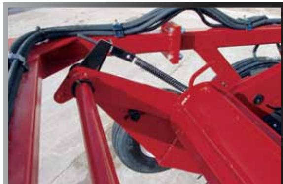
The pick-up head crop roller is adjustable for height and tension.
