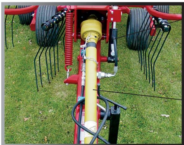
The adjustable front cylinder allows users to fine tune pitch the rake
