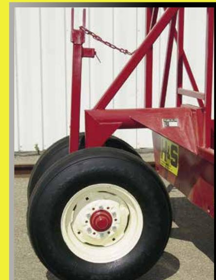
H&S bunks feature a 90° turning radius with tricycle front end, 6 hole hubs and wheels, and quick hitch tongue.
