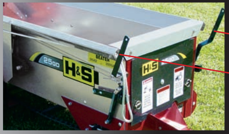
Apron Engage/ Disengage Lever Beater Engage/ Disengage Lever
