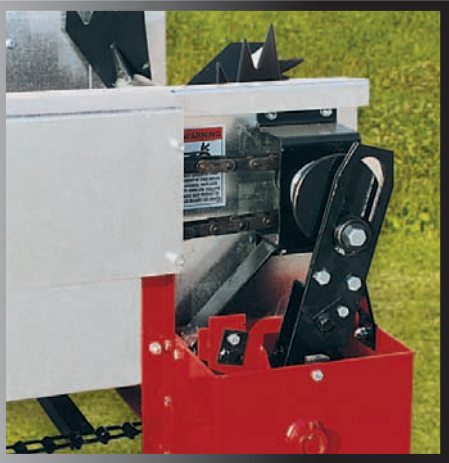
To engage the beater and main apron on Models 50 and 80, lower the control lever.
