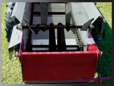
The beater on Model 25 is 20" in diameter and with 8 paddles provides an even spread of material. Shown with optional fine spread pan.
