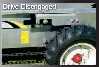
To engage the beater and main apron on Models 50 and 80, lower the control lever.
