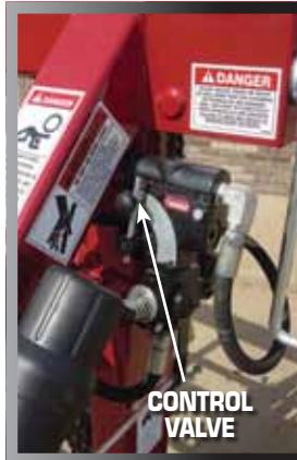
The speed of the tedder reel is hydraulically controlled. Manually adjust the control valve for crop and field conditions.
