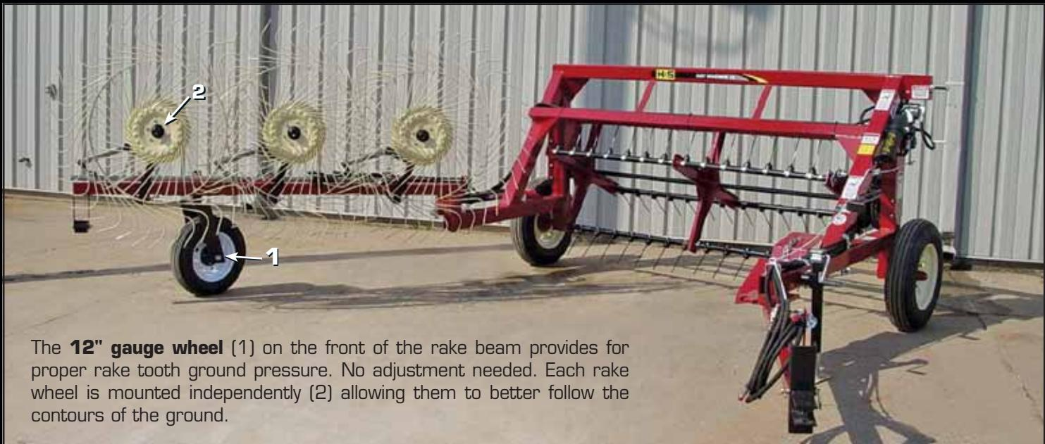
The **12" gauge wheel** (1) on the front of the rake beam provides for proper rake tooth ground pressure. No adjustment needed. Each rake wheel is mounted independently (2) allowing them to better follow the contours of the ground.
