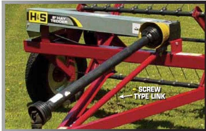
The **screw type link** (below the PTO Shaft) allows for handy and easy height adjustment. Cut hay that has been rained on can be tedded to speed up drying and avoid spoiled hay.
