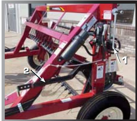
The **hand crank** (1) is for tedder reel height adjustment and the cam lever (2) is used to adjust the aggressiveness of the tedder teeth for a fluffier windrow.
