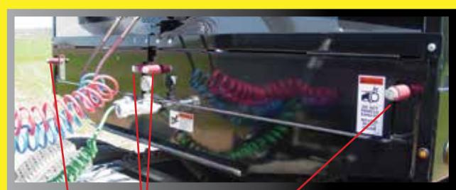
Apron tension adjustment is made by tightening the 4 spring loaded tightener bolts on the front of the box. The spring loaded tighteners maintain tension on the apron during start up and operation.
