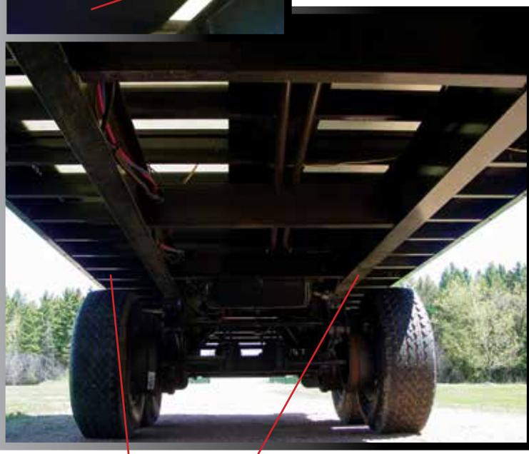
The main frame is made of high quality formed steel 10" I-Beams for the rear and compressed down to 5.13" in the front with full length front gussets.
