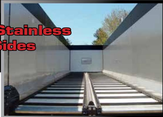
The PL88C OPEN BARREL main apron pintle chain @ 29,900# per strand stays flexible. 2" x 1" x 3/16" formed apron channels are used for the apron cross bars. The floor is 1/2" thick virgin grade solid poly. A stainless steel center between aprons that is formed to eliminate any feed build-up for a complete clean out.
