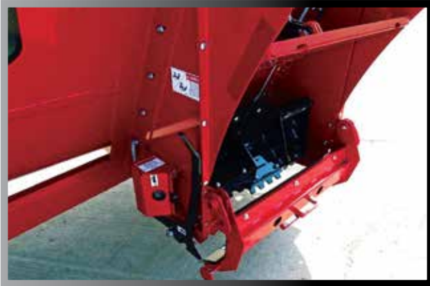
The 5115 features a 3 Section - 30" Expeller with a quick release poly-lined fine spread pan.
