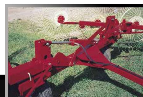
Raking width on the H&S V-rakes can be adjusted to 3 different positions with the pin and fine tuned by adjusting the turnbuckle screw. The hitch jack is used to adjust the windrow width as shown.
