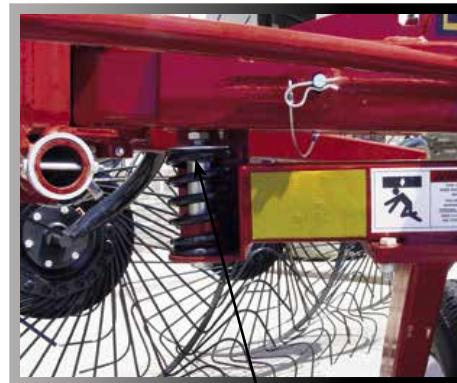
The operator can adjust the fine tune spring to allow proper rake wheel down pressure on each arm of either rake.
