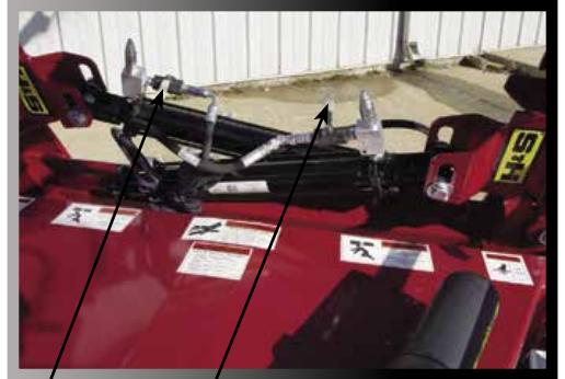
**RIGHT** and **LEFT** side raking is done easily by turning either one of the wing transport valves off.
