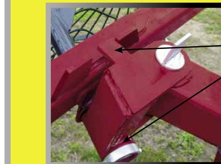
The Rake Arm Pivot Joint provides flexibility for the rake beam in uneven ground conditions unlike most competitors.
