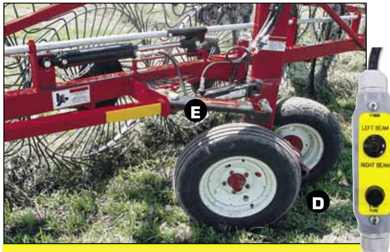
Tandem 6.70 X 15 tires w/rims (D) are standard equipment. X-Series Rakes have a hydraulic adjust beam angle (E) as standard equipment.
