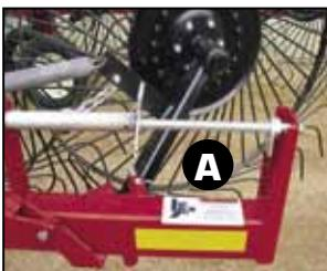
Each rake beam has a screw adjustment (A) for the rake wheel ground pressure allowing the operator to fine tune for various conditions.
