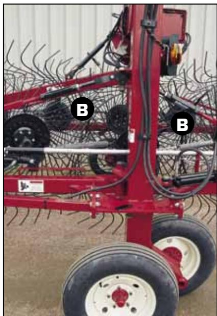
Two turnbuckle adjustments (B) on the support rods of each rake beam adjust to keep the rake beam level.
