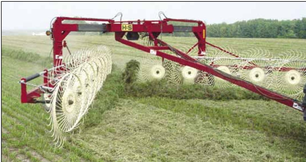
The H&S X-Series Rakes feature a highly maneuverable short turning radius, no caster wheel design, and an overhead frame design for high volume capacity of Crop.
