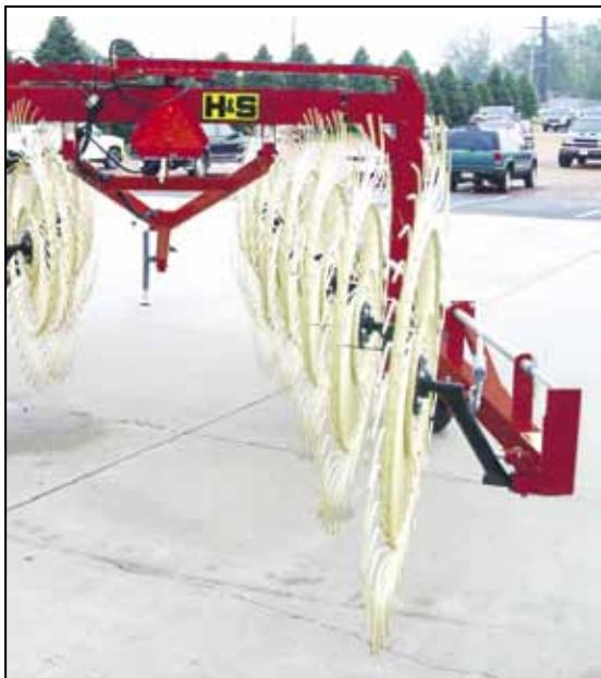
Like all H&S Rakes, the X-Series Rakes have a proven ground pressure system and rake arm design. The X-13 & X-15 Rakes have 100% coverage, there is no need for center kicker wheels. The 3 wheel extension can be locked up if not needed. All models of the X-Series Rakes also feature one side raking with either side.
