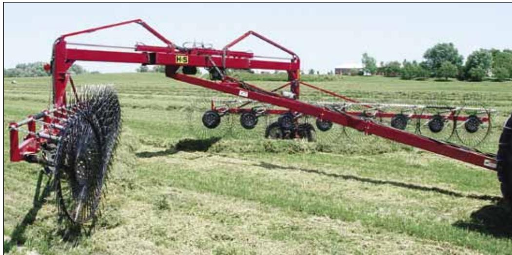
The H&S HDX Series Rakes feature a highly maneuverable short turning radius, no caster wheel design, and an overhead frame design for high volume capacity of crop.
