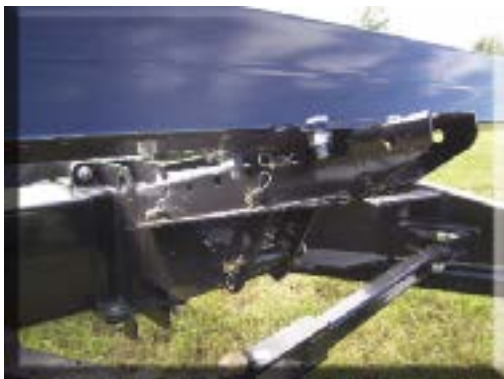
Adjustable upper support tube for flexibility when mounting heads
