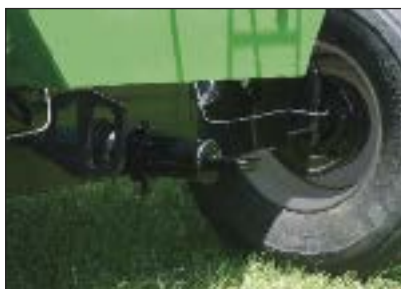
One piece reach pipe for pull through rear hitch design and safety chain support
