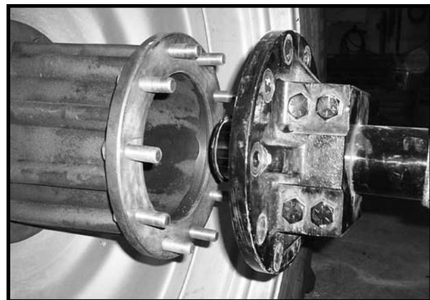
3. Bolt the Hub Spacer to the tractors dual using (8) new Hex Hd. Bolts (specific to tractor model) and tractors original washers. Remove starter studs and install the last 2 Hex Hd. Bolts and tractors original washers.
