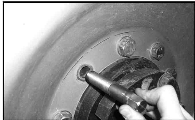
1. Insert 3/4" x 2.875 studs into Hub Spacer using nuts to pull them in.
