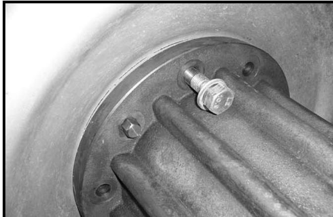
2. With proper hydraulic jack, lift tractor until weight is off dual wheel but still touching ground. Remove top and bottom lug bolts on the tractors dual. Insert 2 alignment studs (13919-95). Remove the remainder of lug bolts.
