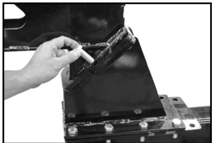
8. Install tank receiver assy onto cross tube mount using (4) 5/8" bolts and nuts.
