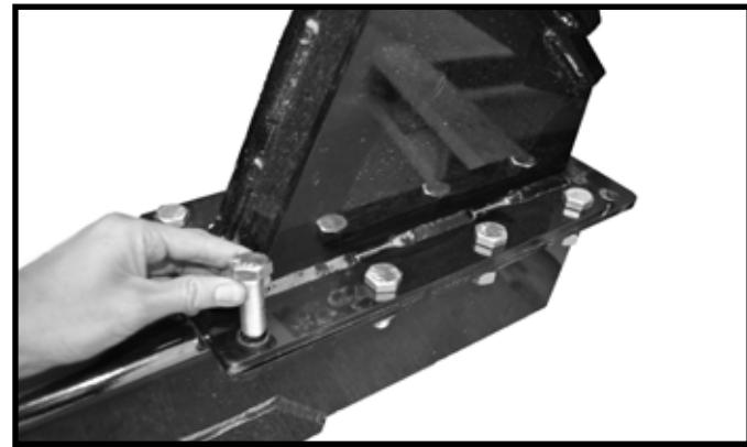
5. Install cross tube using (4) 3/4" hex hd bolts, nuts and washers. Leave the bolts loose until tank receiver is aligned and bolted to tank saddle.
