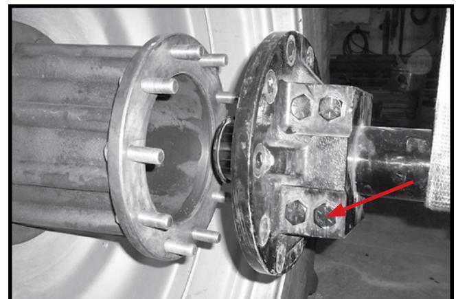
9. Line up slots on bottom of receiver to slots on front of tank assy. This will vary depending on size and type of tractor and wheel size/spacing. Install (4) 1/2" bolts, nuts and washers.
