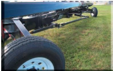
*Steering linkages with ball joints for smooth steering of rear axle. Located on side of main frame, also allows increased ground clearance.*
