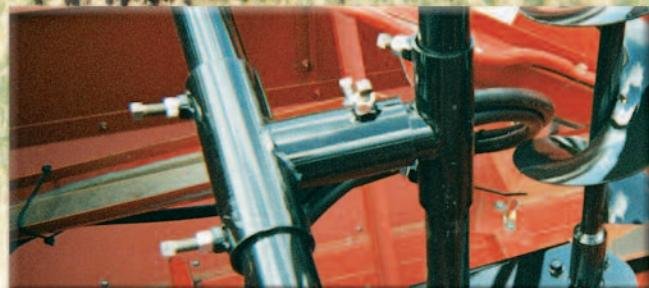
Set screws allow for infinite adjustment to maximize grain holding capacity.
