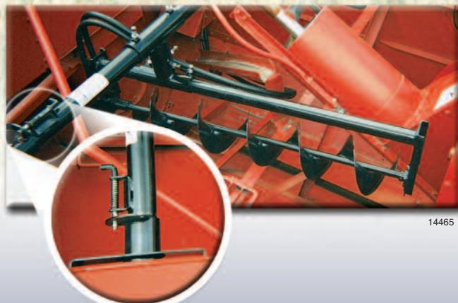
Quick release pivot to lower to transport position in seconds.
