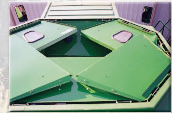
Quick and easy fold down of extension for lower transport height
