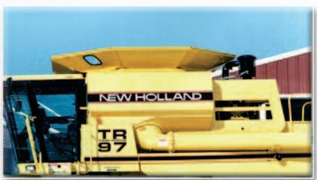
Folded configuration for Caterpillar, New Holland and Gleaner extensions, regular and large capacity models fold the same.
