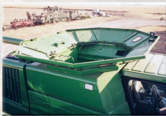
3" formed channel frame on John Deere and Case IH provide unmatched strength and stability.
