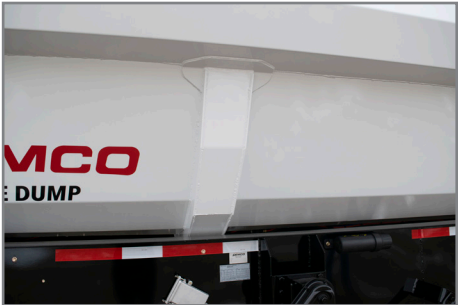
Tub Supports 3 outer tub supports to increase strength
