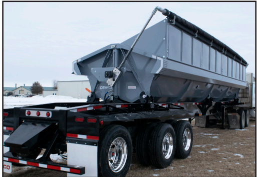
High Capacity Kit 34' Tub - 37.9 Cu. Yds., 37' Tub - 41 Cu. Yds.
