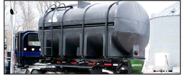
Black plastic liquid tanks eliminate light from reaching the interior contents preventing algae and microbes growth
