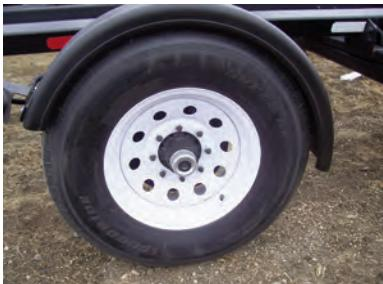
Standard 7,000lbs front and rear torsion flex axles provide smooth and reliable service in the field or down the road! New 16" Highway service radial 10 Ply tires on 8 bolt hubs.
