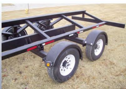
Standard 7,000lbs torsion flex axles with E-Z Lube hubs, front and rear. Standard one axle rear brake. Front and rear fenders are also standard features.
