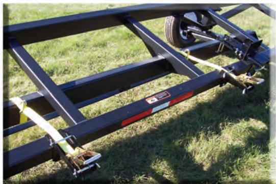
Two fully adjustable ratcheting straps for securing all brands of heads.
