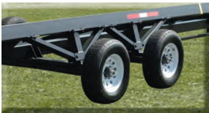
Bolt on ready rear suspension with combination of idler or braking axles.
