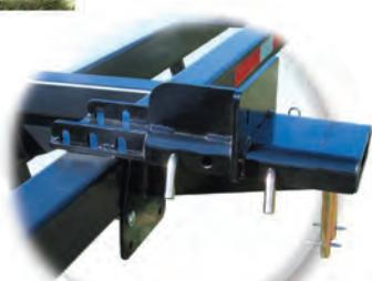
Standard adjustable slider brackets allow the carrying of most heads on the same transport.
