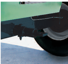
One piece reach pipe for pull through rear hitch design on 450, 550, 650 and 750 models
