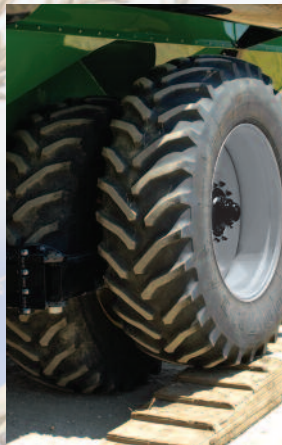
Oscillating inline duals minimize frame stress and field scuffing
