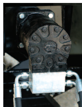
Hydraulic orbit motor for driving horizontal auger eliminates belts and pulleys
