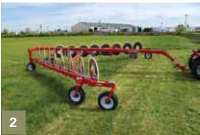
[1] Transport width of 8' [2] Open and close using hydraulics [3] Individually spring loaded wheels prevents digging into the ground [4] All models are equipped with eight wheels [5] Working widths from 32' to 38'.
