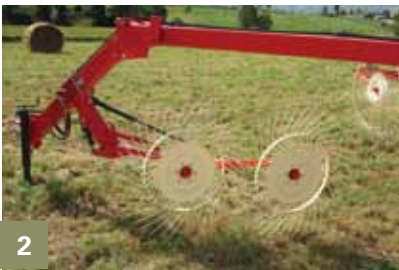
[1] Maximum transport width of 8' [2] Optional center mounted hydraulically operated wheel rake [4] Open and close using hydraulics [5] Four to six stabilization wheels.
