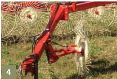
[1] Maximum transport width of 8' [2] Optional center mounted hydraulically operated wheel rake [4] Open and close using hydraulics [5] Four to six stabilization wheels.
