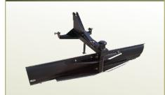
For tractors 30 to 60 hp - available in 7' and 8' widths. Mechanical linkage. Hydraulic adjustment is optional. Cutting edge constructed of high carbon steel, 1/2" x 6".
