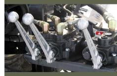
▲ Fingertip hydraulic controls are standard and allows for smooth 4-way tilt, in/out slide and hammer up/down.
