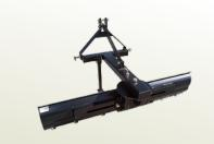
For tractors 20 to 45 hp - available in 5', 6' or 7' widths. 15° vertical tilt on both sides. Cutting edge constructed of high carbon steel, 1/2" x 6".
