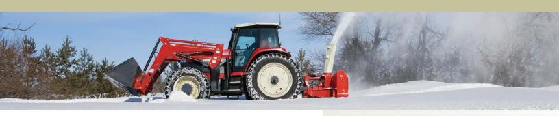
**Model 960** - 96" (2.4 m) cutting width, 3-point hitch Category II / III For tractors 90 - 125 hp
