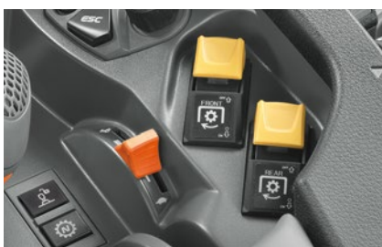
PTO engagement for front/rear PTO.
