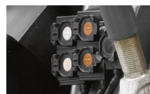
When a front linkage is installed, two hydraulic valves and one free-flow return line are available the front. Ideal for front-mounted equipment.
