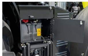
The battery is conveniently positioned above the right-hand access ladder.
