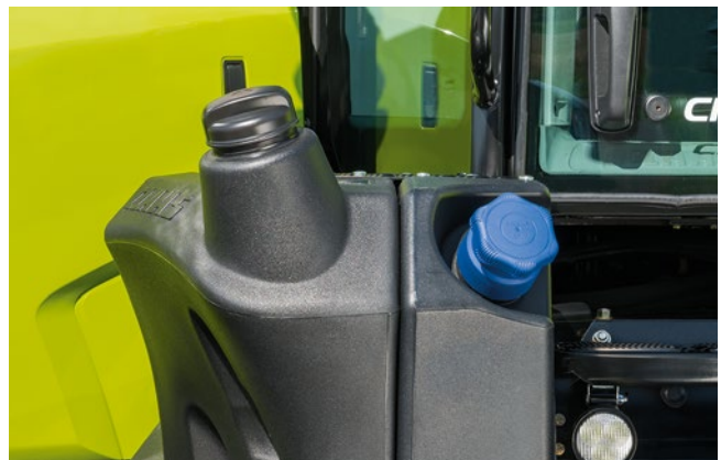
120 gal fuel tank with integrated 11 gal urea tank.
