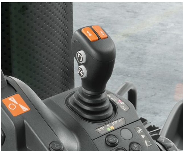
Optional right-hand reverser on the ELECTROPILOT joystick.
