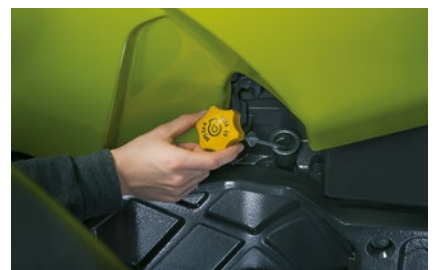
The oil can be checked and topped up when the bonnet is closed.
