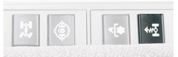
Switch to activate front axle suspension.
