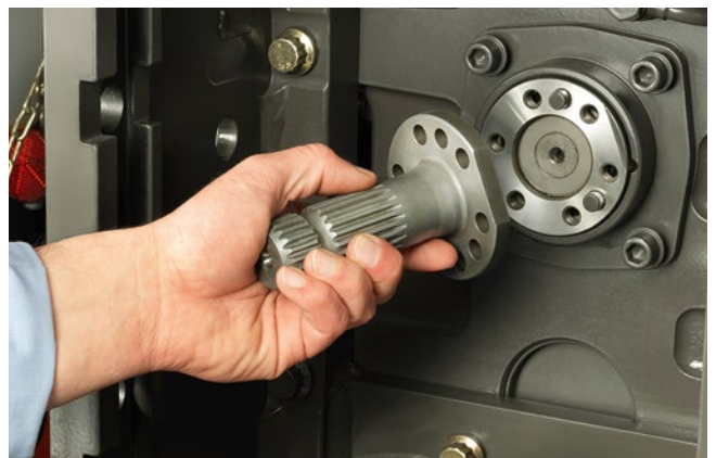
The PTO stub can be changed easily.
