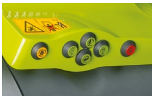
External controls for the rear linkage, PTO and one freely selectable spool valve.
