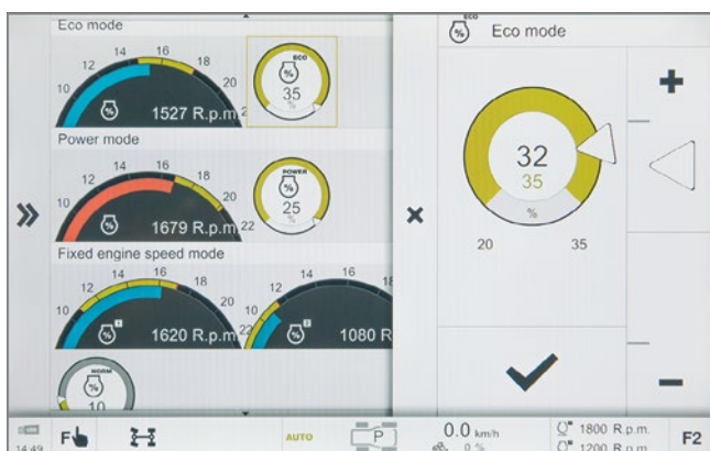
Engine droop setting for "Eco" and "Power", and the engine speed memory.
