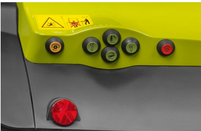
External controls for rear PTO.
