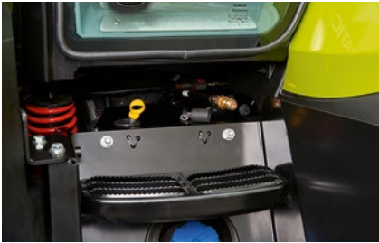
Compressed air connection on the left side of the access steps.
