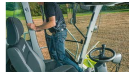
The seat contact switch automatically switches off the front attachment and main drive.
