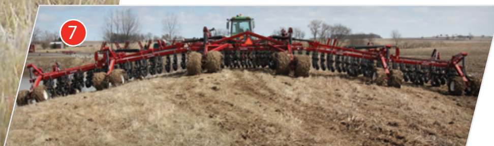
525 - 60' and 70' primary wings flex 24" down and 37" up at the tip
