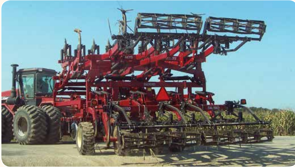
■ Wing fold models fold flat. Working widths up to 22 ft. transport and store easily at 12'6" ft.
