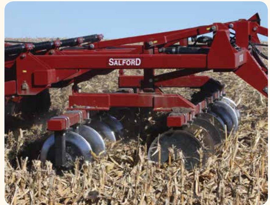
■ Independent "overhead" gangs and individually mounted blades for maximum residue flow
