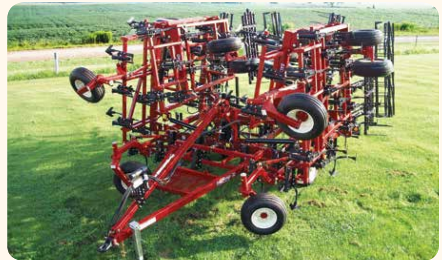
■ Model 700 C-Shank, wing fold cultivator with the 'Land Hugger' option.
