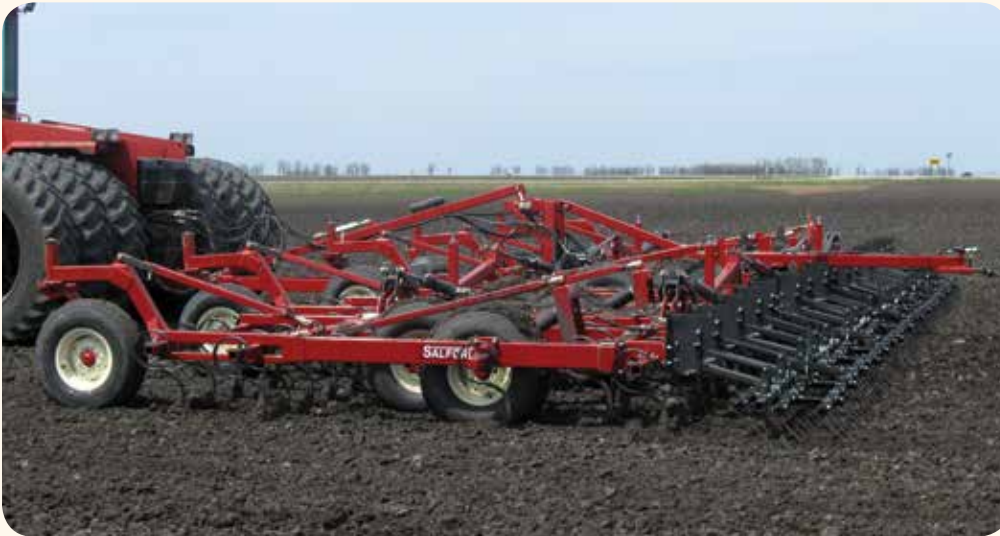
■ 700 S-tine cultivator with tow hitch. Durable 4"x 6" mainframe with reinforced 2.5" square tine bars
