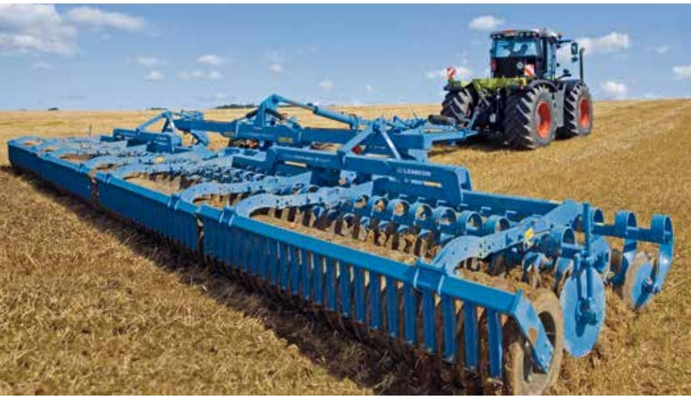
The Helidor compact disc harrow from LEMKEN uses two rows of discs individually mounted to leaf springs. This system provides a uniform cultivation depth, whilst allowing individual discs to ride over stones when necessary. During stubble cultivation the discs ensure soil and vegetation are evenly and intensively mixed.
