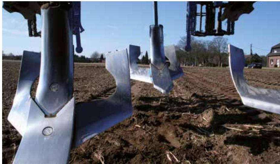
The new Kristall compact cultivator from LEMKEN can be used for both shallow and medium depth work in several stages. The initial shallow cultivation involves the specially shaped TriMix stubble shares working volunteer grain and organic mass into the soil across the entire width and close to the soil surface. The volunteer grain remains in the upper layer of soil where it will quickly germinate.
