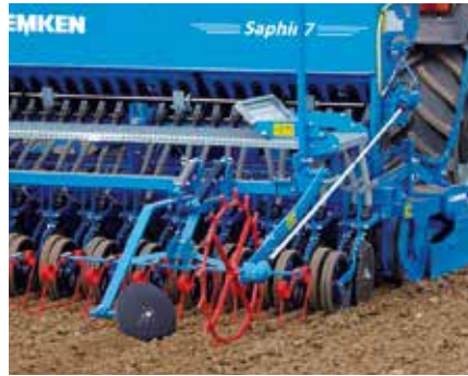
Maintenance-free universal-shaft drive
